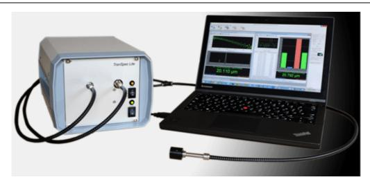
The **TranSpec Lite** film thickness gauges use the white-light interference phenomenon for non-contact and non-destructive layer determination of transparent single or double layers in the range of around 0.8 to 120 micrometer (depending on the model). The TranSpec Lite instruments are designed for manually performed, but even though high-precise measurements in the lab.
